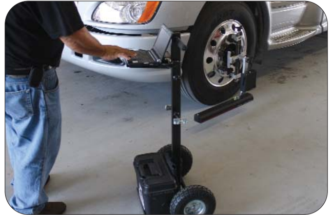
The technician mounts the QTAC diagnostic equipment on the tractor and completes the check in under 5 minutes.
