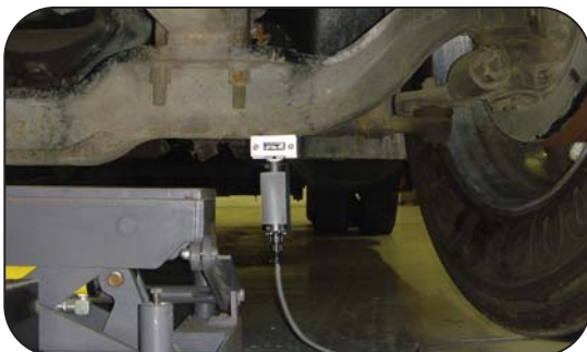
2. A sensor measures wheel vibration
