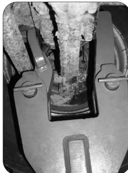
THE 404080 IS DESIGNED TO SLIDE BETWEEN THE AXLE AND TIE ROD ON HEAVY DUTY AXLES.
