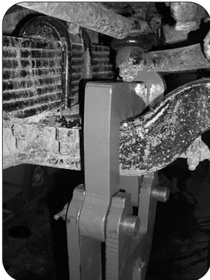
THE 404076 RESTS ON TOP OF THE AXLE AND UNDER THE STEERING ARM.
