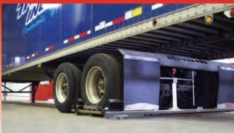
Figure C - With the Bee Line Laser Tandem Aligner, offset axles and axles with uneven spacers are set perfectly at 90° to the centerline of the vehicle. Additional axles are then simply set with a tram gauge.
