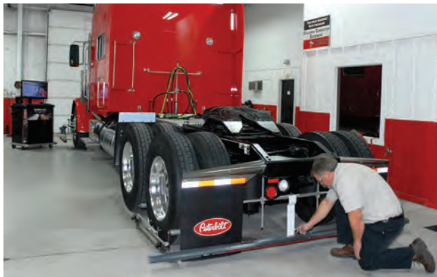
Set the rear axles with computer accuracy using the 22000 Rear Axle Aligner.
