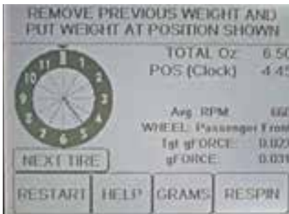
3. The touch screen indicates the position and how much weight should be placed on the wheel.
