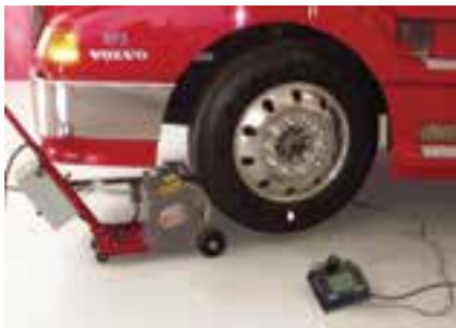
1. A spinner brings the wheel up to speed.
