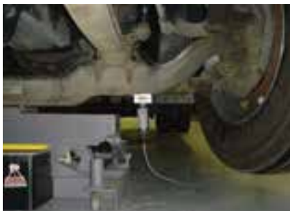
2. A sensor measures wheel vibration
